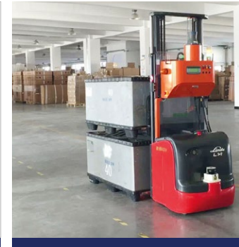
Kollmorgen System Laser Guided Stacker Linde Forklift AGV
