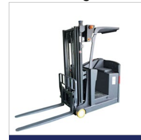
Laser Guided 3m Counter Balance Forklift AGV
