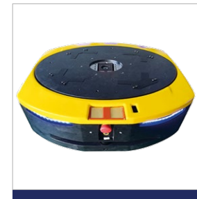
CE Complied 600kg Payload Standard ELFIN Warehouse Logistics AGV Robot
